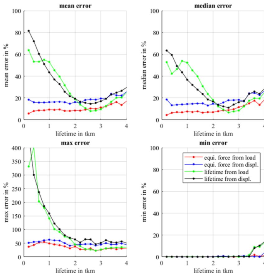
Fig. 6. Errors of the predicted lifetime values compared to the exact RCLE top left: mean error top right: median error bottom left: max error bottom right: min error
