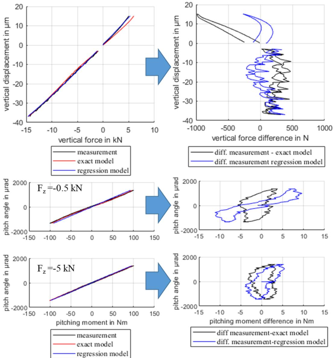
Fig. 7. Comparison of the experimentally measured and calculated carriage displacements
