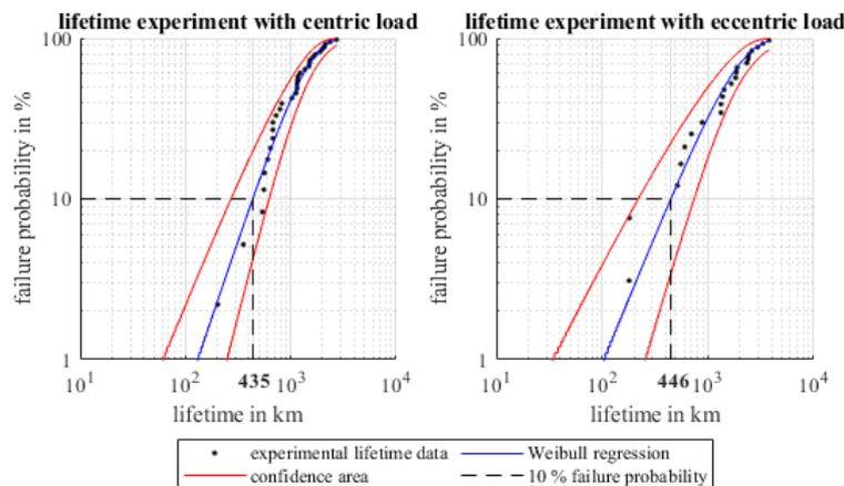
Fig. 1. left: Weibull-analysis for a centric load, right: Weibull-analysis for an eccentric load
