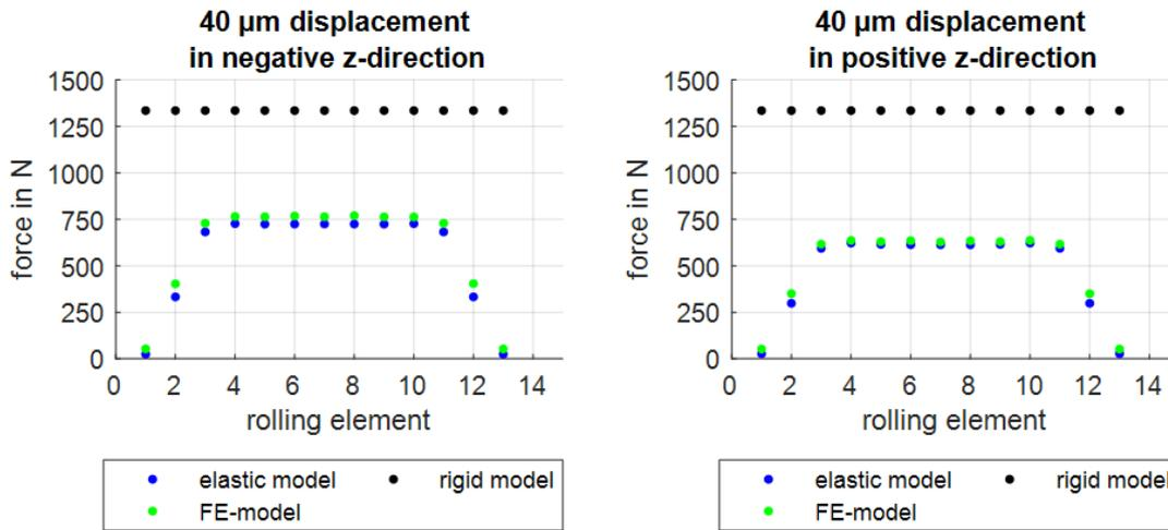
Fig. 3. Distribution and comparison of the calculated rolling contact forces
